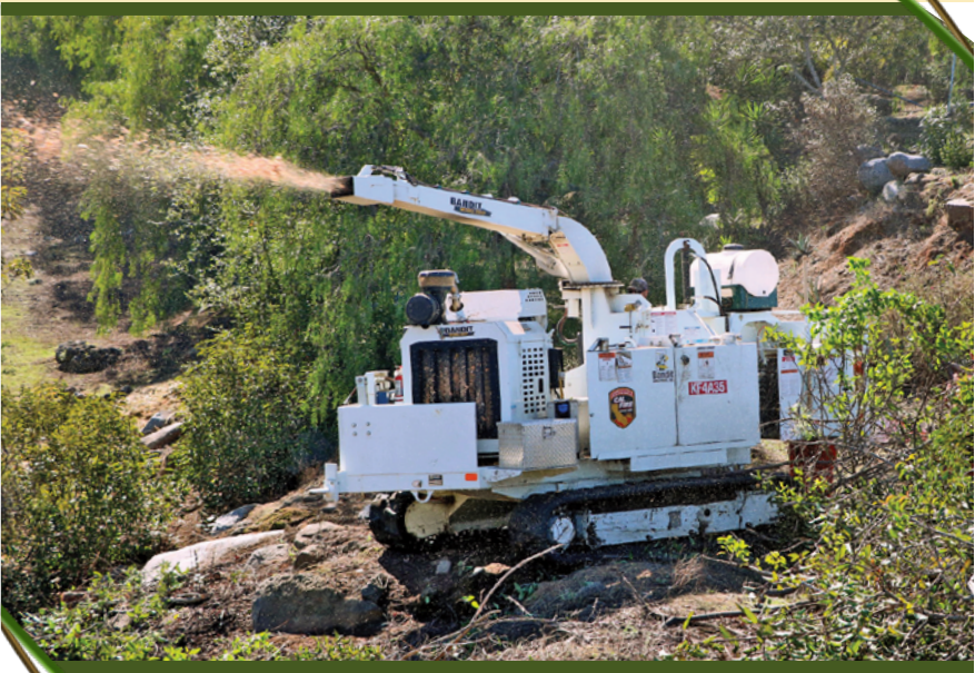
Chippers are an important part of CAL FIRE's fuels reduction work. Both tracked and tow chippers are used where hand thinning projects are being completed.
